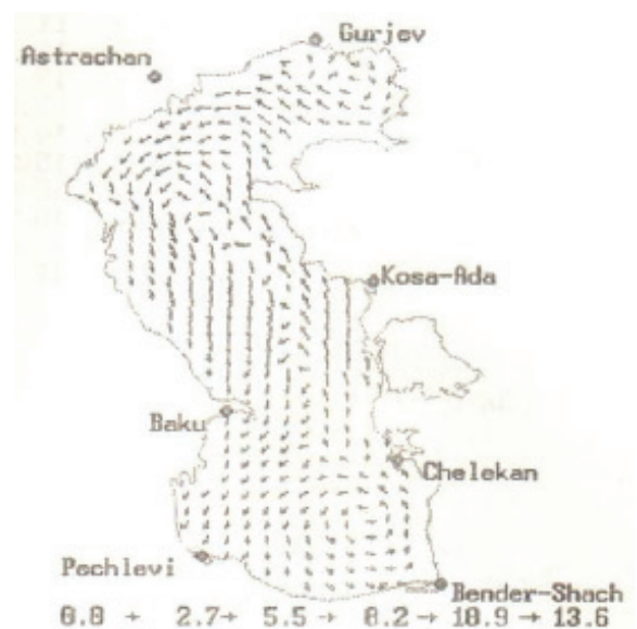
Figure 3. Velocity fields under influence of the average annual data at the surface.
