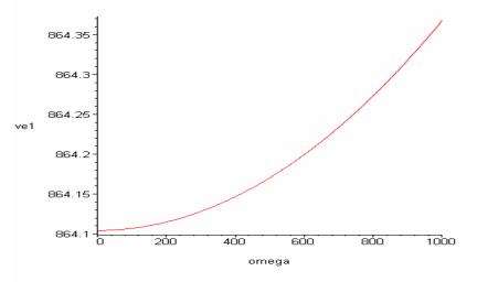
Fig.1. Propagation velocity of first kind viscoelastic wave in saturated by liquids porous media
