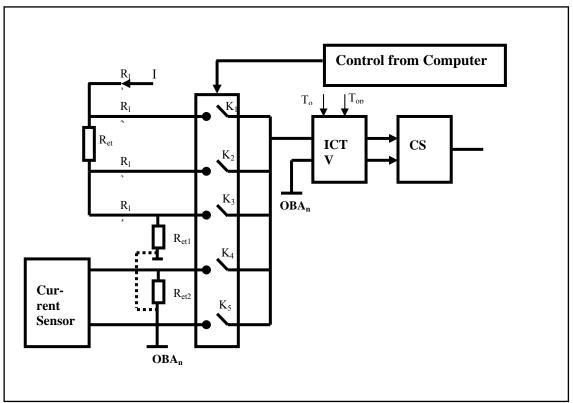
Fig. 1. The scheme of measurement of resistance TRT and current signal.
