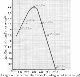
Fig. 4. Dependence of signal value on the length of current electrode  $\delta$ ,  $\lg U_s = f(\delta)$ .
