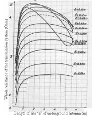
Fig 3. Dependence of the whole resistance of the transmission system on the length of "a" of various  $\delta$ , z = f(a),  $\delta = var$ .
