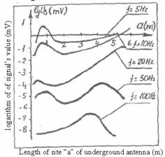
Fig. 5. Dependence of signal value on the length of site "a" at the various frequencies  $\lg U_s = f(a)$ ,  $f = \operatorname{var}$ .
