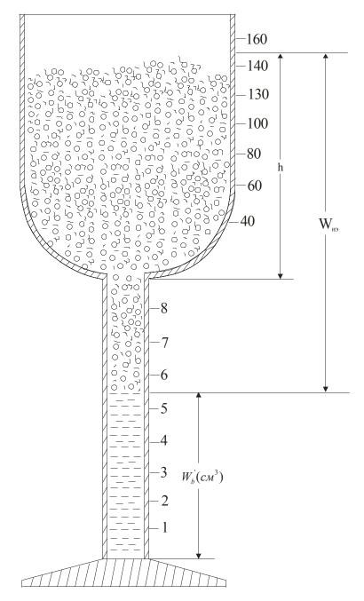
Figure 1. Graduated vessel for sedimentation
