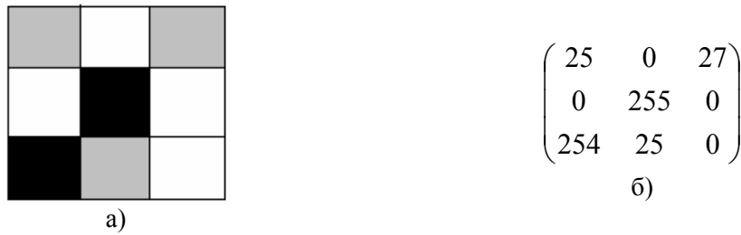
Picture1. Fragment of the scene 3x3 (but) and numerical values level sulphur in pixel (b)
