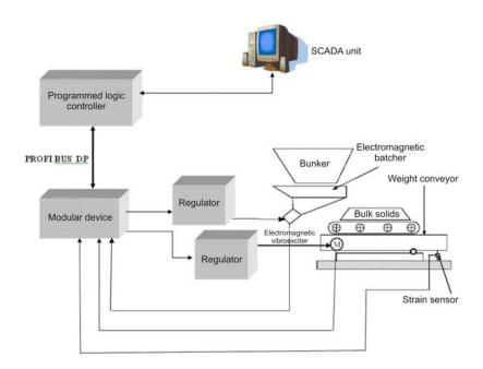
Fig. 1. Control system vibrating injector.
